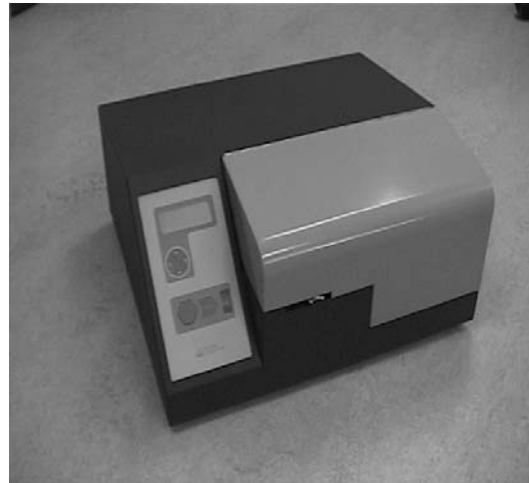
Fig. 7 The field deployable biosensor analysis system
