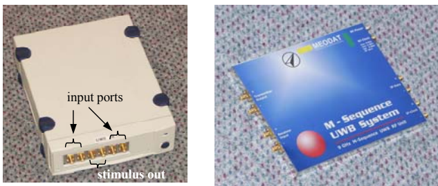
Figure 5. Example of the basic radar (left) and a RF-Module (right).
